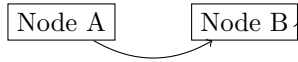
Figure 4: The points-to relationships between heap objects in test_interp . This example is exceedingly simple, as it was designed with two separate functions (to test our interprocedural support), one for pushing and one for popping, treating the linked list as a stack.
